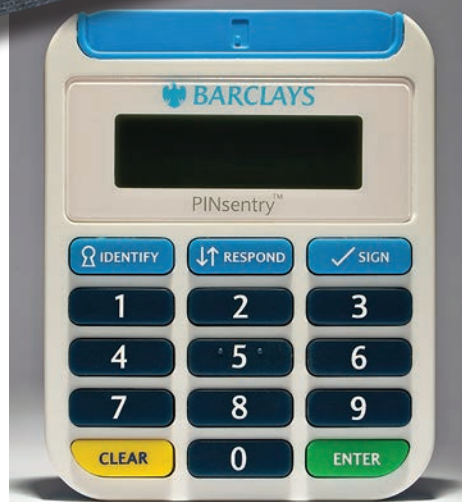
A Chip Authentication Program (CAP) card reader used in conjunction with EMV cards.
